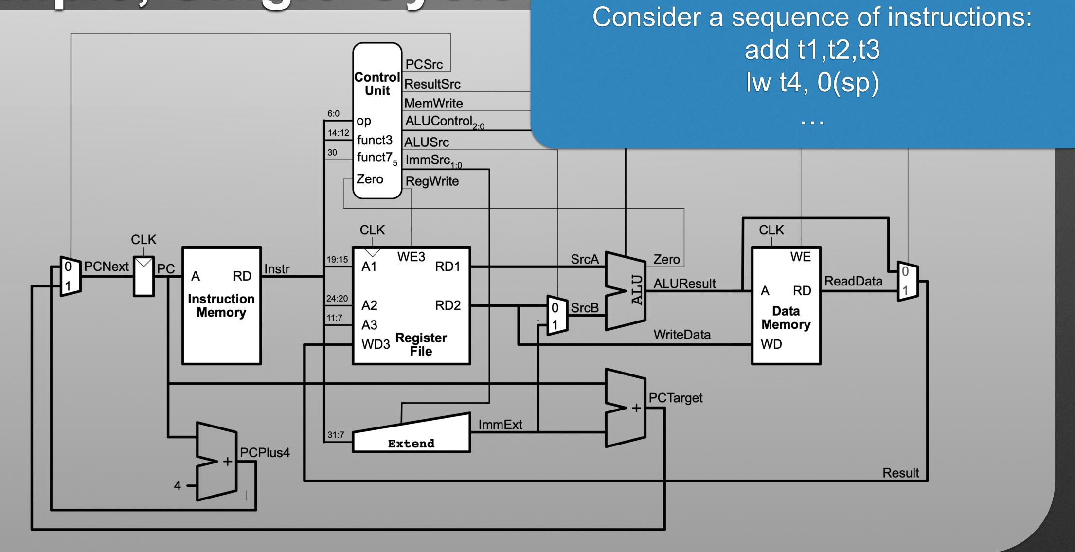
Simple, Single-Cycle PISC-V Computer Consider a sequence of instructions: add t1,t2,t3 **PCSrc** Iw t4, 0(sp) Control ResultSrc MemWrite ALUControl<sub>2:0</sub> ALUSrc ImmSrc<sub>1:0</sub> RegWrite CLK **CLK** CLK WE3 WE SrcA Zero RD1 Instr RD ReadData **ALUResult** RD Instruction Memory Parts are "Idle" (done with their role in the instruction) most of the time. This is inefficient! Result
